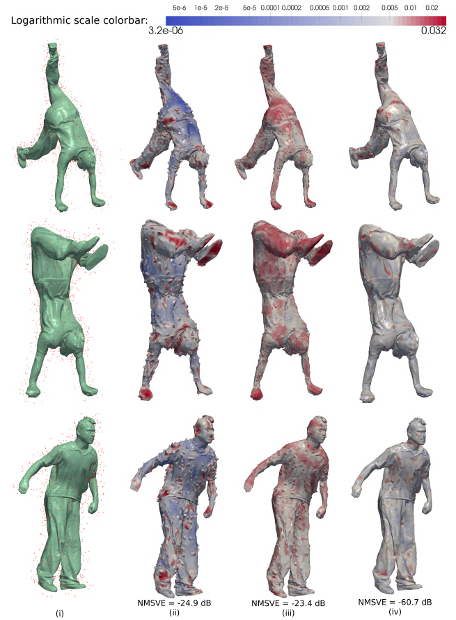
FIGURE 9. Outlier removal on the Handstand animation model: (i) 20% noisy points, (ii) output of WLOP, (iii) output of Static RPCA, (iv) output of RPCA applied to the time-varying point cloud matrix (DRPCA). The proposed outlier removal method successfully identifies and removes the outliers even in the extreme case where 20% of the points can be considered as outliers, randomly distributed over the range of 1/50 of the bounding box's diagonal length.
